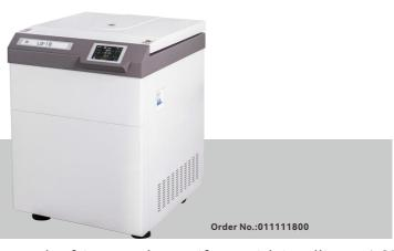
The LG-18 is a multipurpose floor standing high speed refrigerated centrifuge with intelligent LCD touch screen. Equipped with RFID rotor identification technology and three-axis gyroscope real-time monitoring technology. It can spin up to 18000 rpm/31405 xg, 15 rotors for choice to meet different centrifugal needs.
